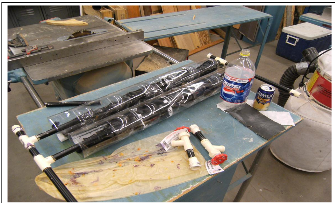
The soda bottle/pop can solar water heater constructed for the Recycle Expo. The valves in the foreground were added to the heater the next day.
